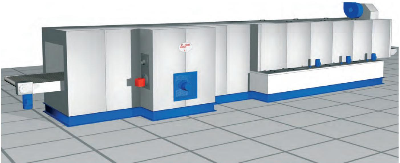
"Three-phase range – Methane and/or GPL burner – Maximum temperature of the degreasing bath 60 °C – Maximum temperature oven 100 °C"
