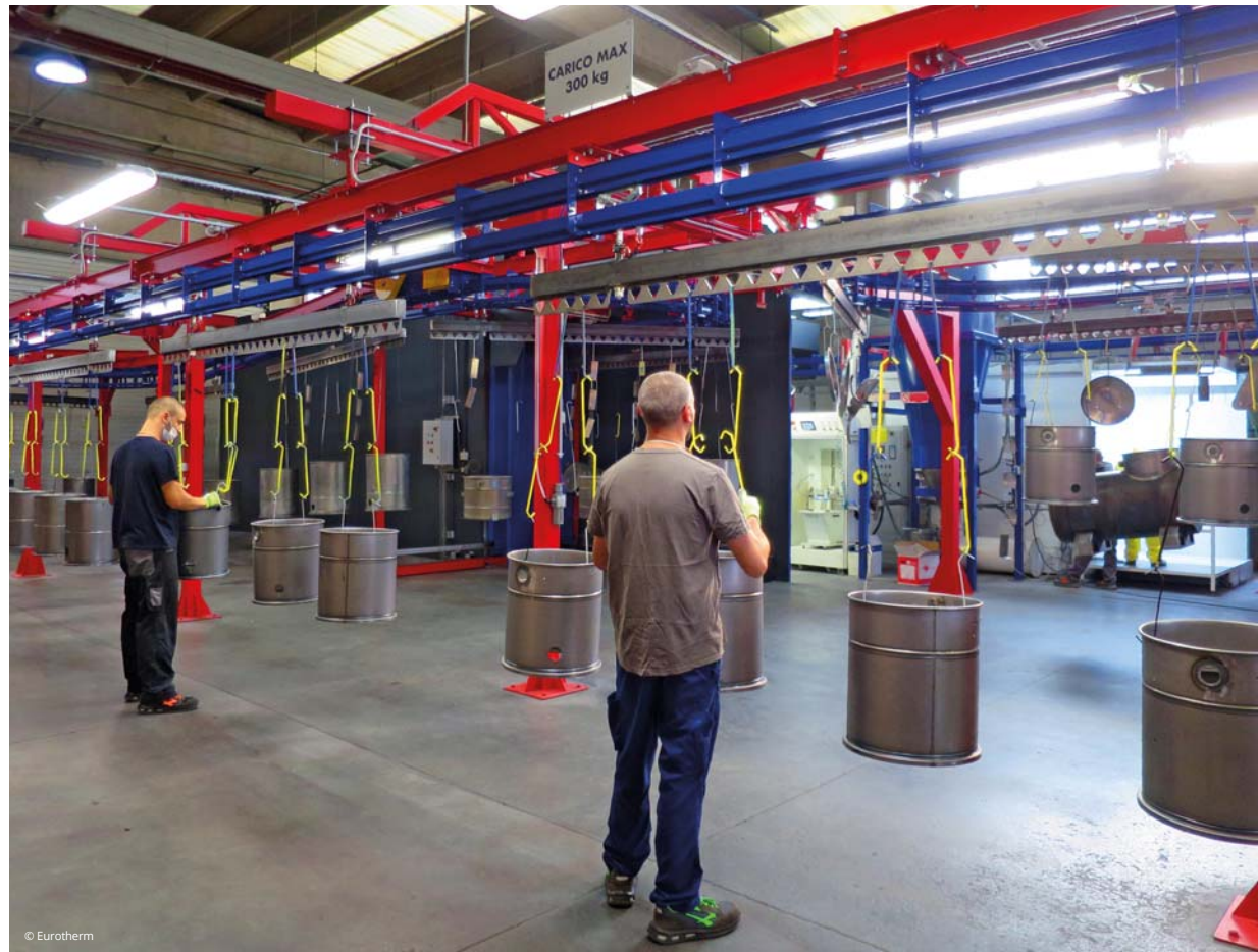
Loading operation: the racks number has been increased from 33 to 39.
