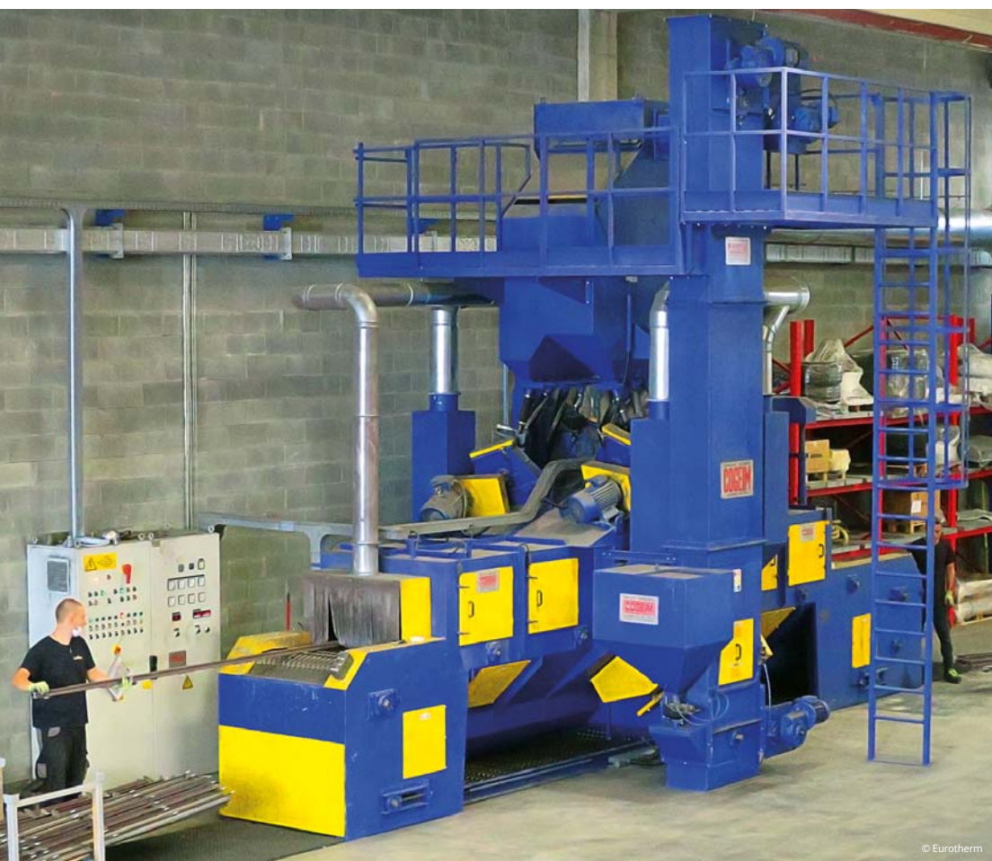
Sandblasting plant with stainless steel grits.
