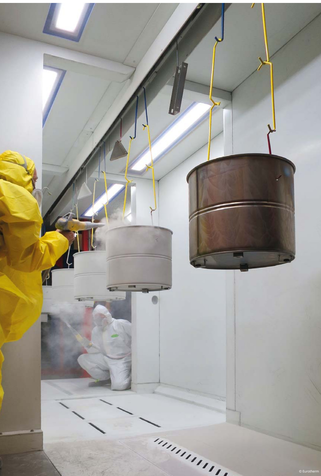
Application of the powder top coat.
